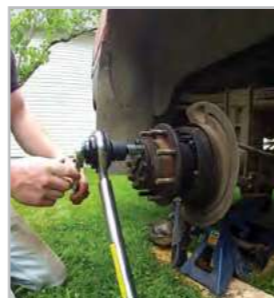
Torque multiplier used for lug nuts
