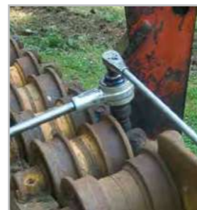
Torque multiplier used on tracks
