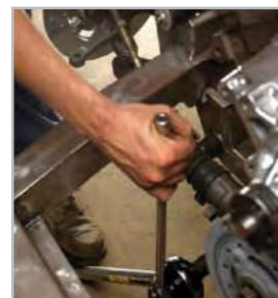
Torque multiplier used in inaccessible areas
