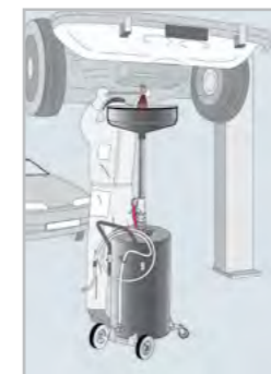
Used oil being drained from vehicle in an automotive workshop
