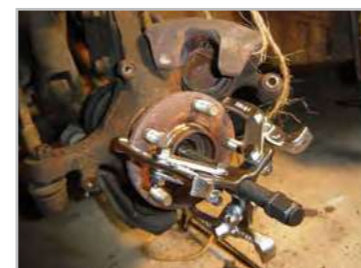
3 Jaw Puller used for removing tyre hub
