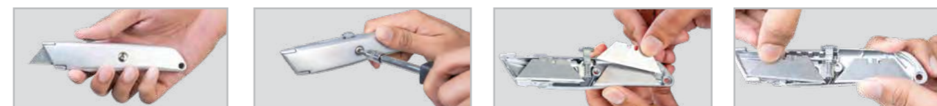
Press the lever down & push forward to load blade
