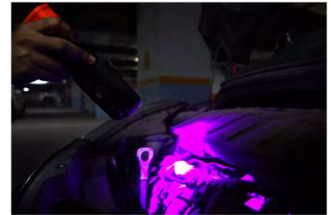
UV light for detecting engine oil leakage, gas leakage, crack in welding jobs in industrial, automotive, HVAC applications
