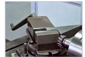
Milling Machine Vice being used to hold a job for milling operation
