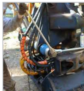
Torque multiplier used for machine nut tightening
